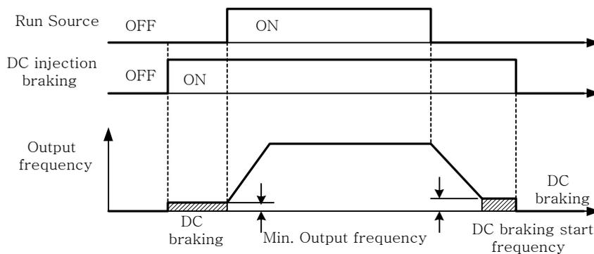
Fig 43 Time chart for DC injection braking command
