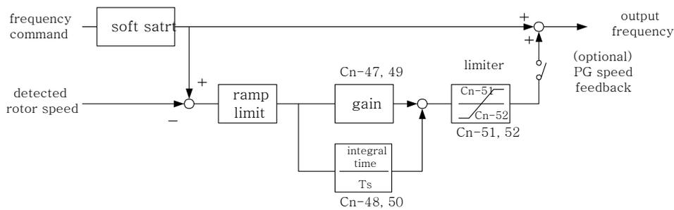
Fig 44 PG speed control block diagram
