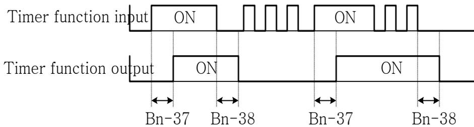
Fig 16 An operation example of timer function
