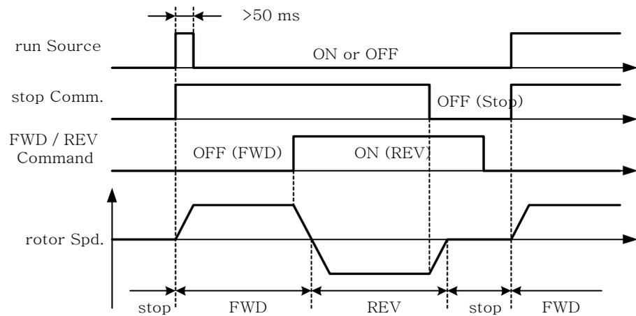
Fig 39 Operation sequence in 3-wire mode
