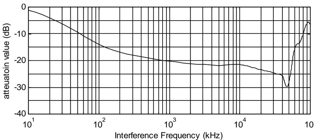
Frequency attenuation characteristics (10 windings case)
