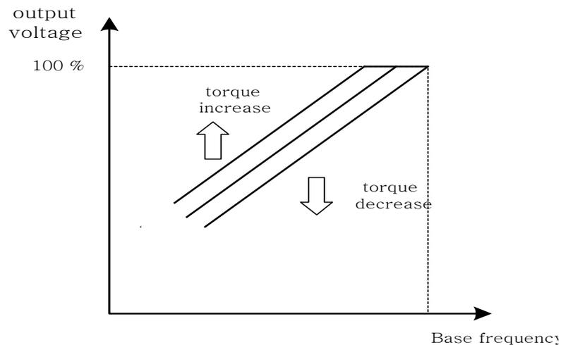
Fig 13 Adjust the auto torque boost gain Bn-11 to increase the output torque.
