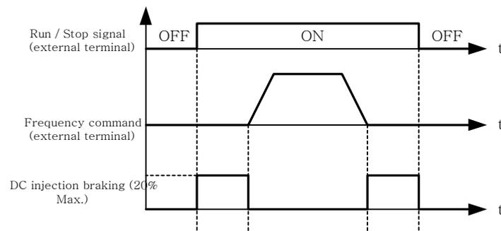
Fig 36 Zero speed braking operation selection
