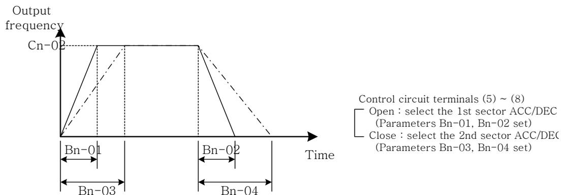
Fig 11 Acceleration and Deceleration time
