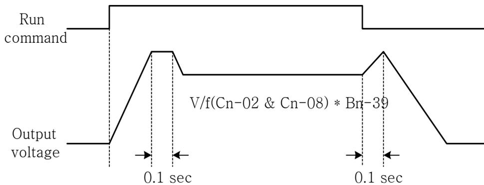
Fig 17 Time chart for energy-saving operation
