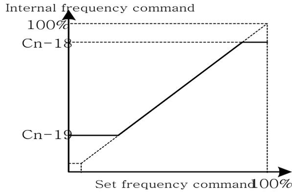
Fig 22 Upper and lower bounds of the frequency command
