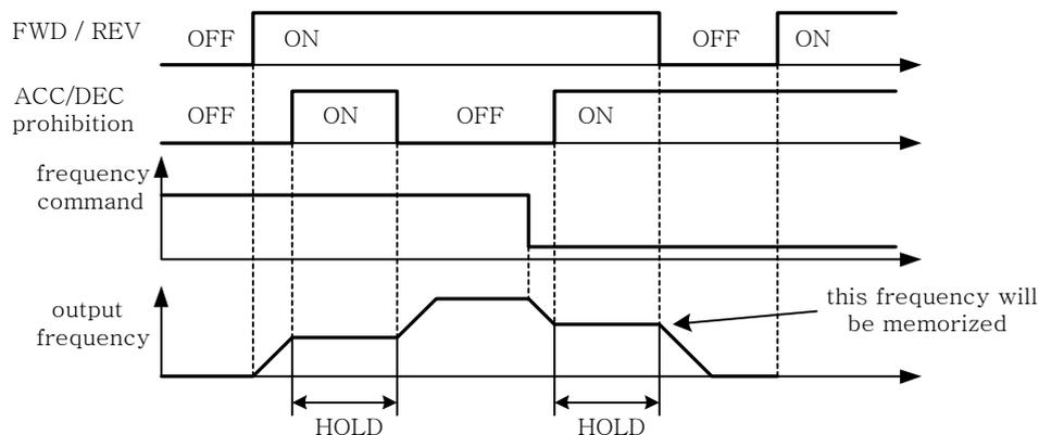
Fig 42 Acceleration and deceleration ramp hold
