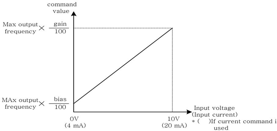
Fig 12 Analog input gain and bias
