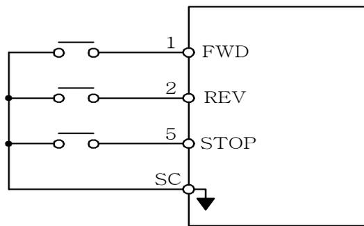
Fig 40 2-wire mode connection diagram
