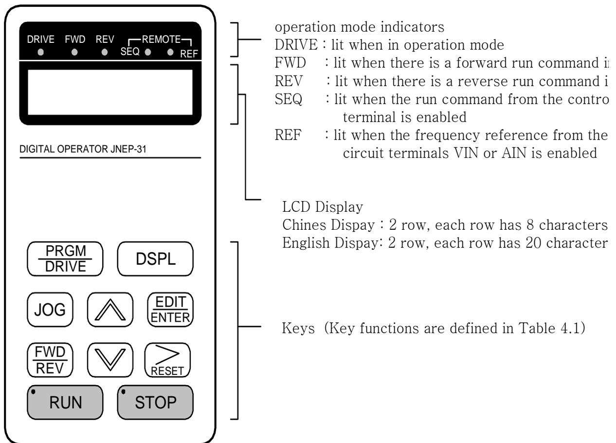
Fig 10 LCD Digital operator component names and functions
