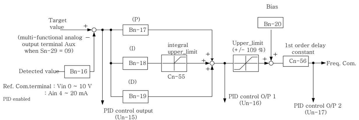
Fig 14 Block diagram for PID control in inverter
