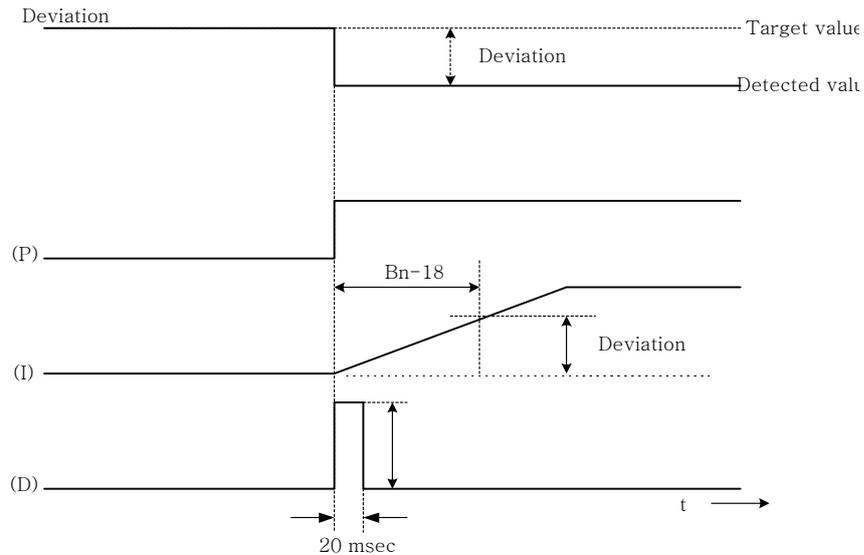
Fig 15 Response of PID control for STEP-shape (deviation) input
