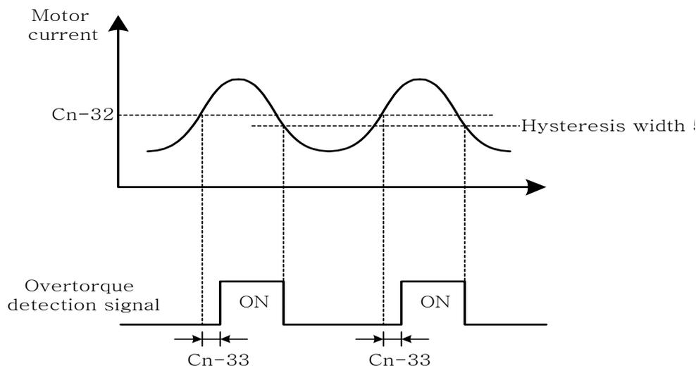
Fig 26 Time chart for overtorque detection
