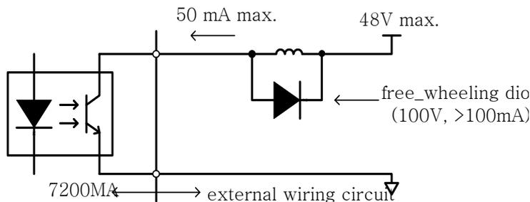
Fig 4 The Optical-couplers (open-collector) connect to external inductive load
