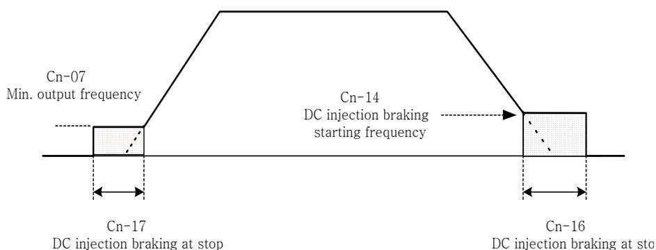
Fig 21 DC injection braking time chart
