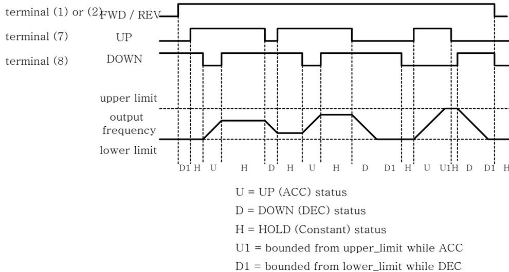
Fig 45 Time chart of output frequency through the external multi-function input terminal ① and ⑧.
